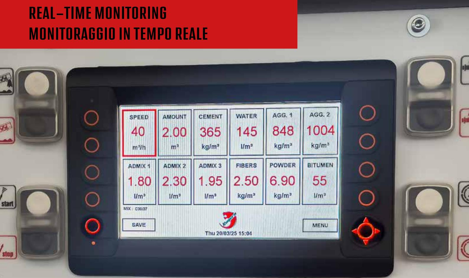
The G Series electronic management system ensures intelligent and automated control of the entire production process. Thanks to an intuitive interface and an advanced PLC, the plant constantly monitors dosing and automatically corrects any deviations, ensuring optimal quality and repeatability.
